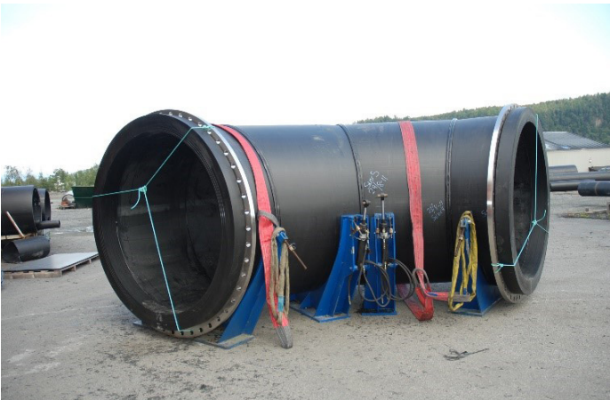
Fabricated 90 deg bend fitting for OD2000 mm
